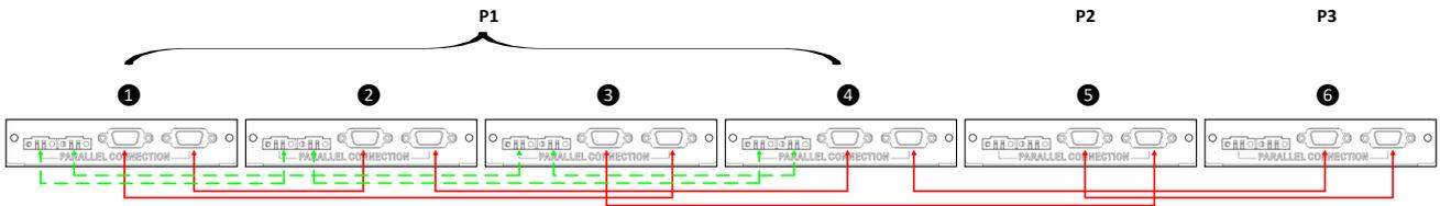
Three inverters in one phase, two inverters in second phase and one inverter for the third phase:
