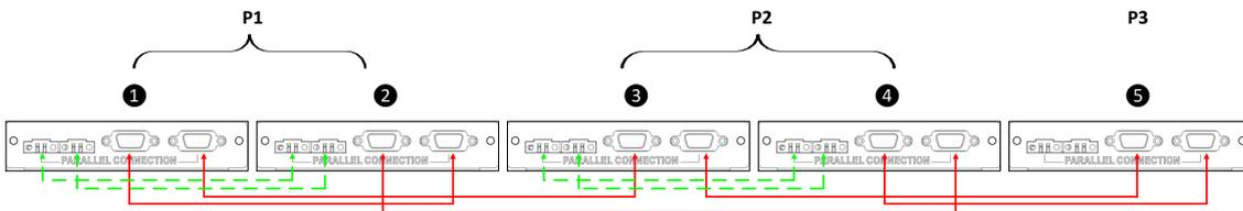
Two inverters in one phase and only one inverter for the remaining phases:
