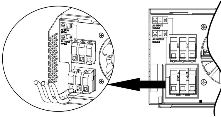
5. Make sure the wires are securely connected.
