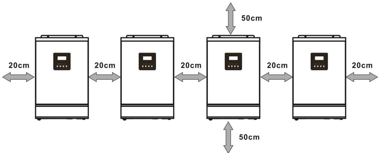
**NOTE:** For proper air circulation to dissipate heat, allow a clearance of approx. 20 cm to the side and approx. 50 cm above and below the unit. Be sure to install each unit in the same level.
