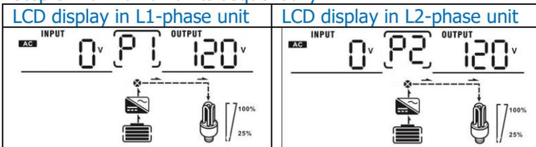
Step 4: Switch on all AC breakers of Line wires in AC input. If AC connection is detected and two phases are matched with unit setting, they will work normally. Otherwise, the AC icon will flash and they will not work in line mode.
