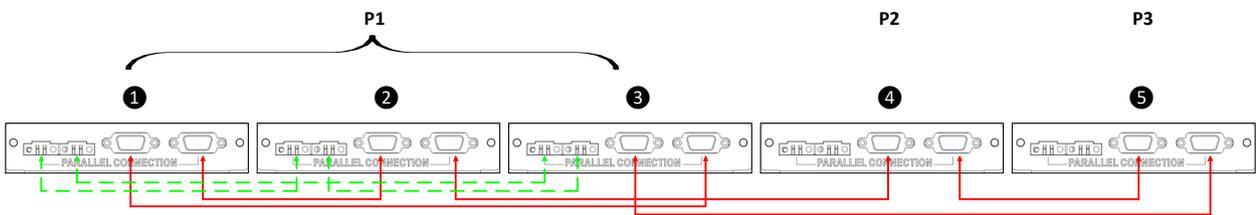
Two inverters in two phases and only one inverter for the remaining phase:
