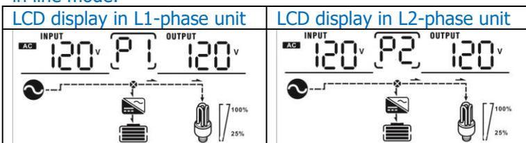
Step 5: If there is no more fault alarm, the system to support 2-phase equipment is completely installed.
