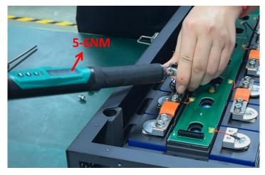
2. Because our box is pre-assembled, check whether the positive and negative screws and the circuit breaker screws are locked before assembly.
