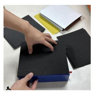
Step 4. Put on the epoxy boards, and put the cells one by one, each cell has one epoxy board between
