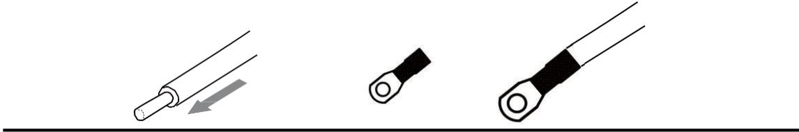
**Step2.** Cross the battery cable through the battery port. Connect battery cable to battery terminal
